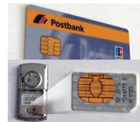
IC chips embedded in a Smart card and a mobile phone SIM card
